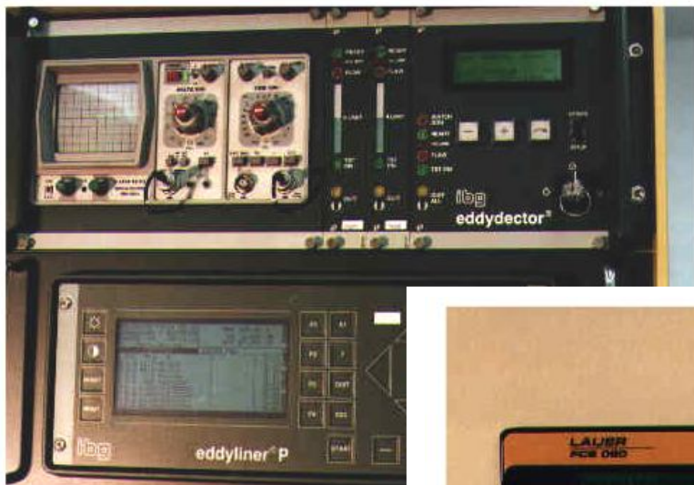
Operation of the test system via softkeys and clear text display.
