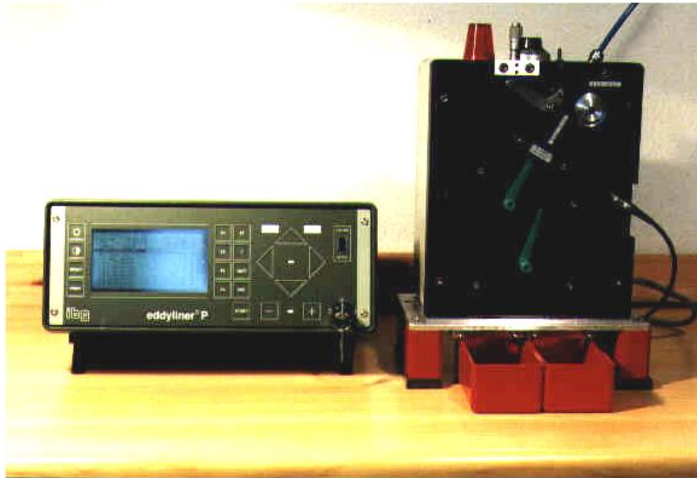
General view of test system with eddyliner®P and sorting unit, P/N 11031. Blue flexible tube for feed of parts.
