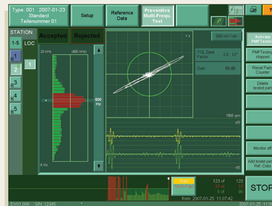
eddyvisor ®SC with crack detection
