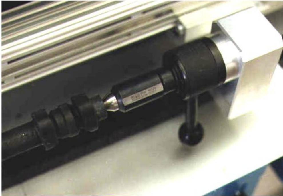
Easy positioning of the test part by quick-clamping element (¼ rotation of the handle to loosen the spring-loaded top).
