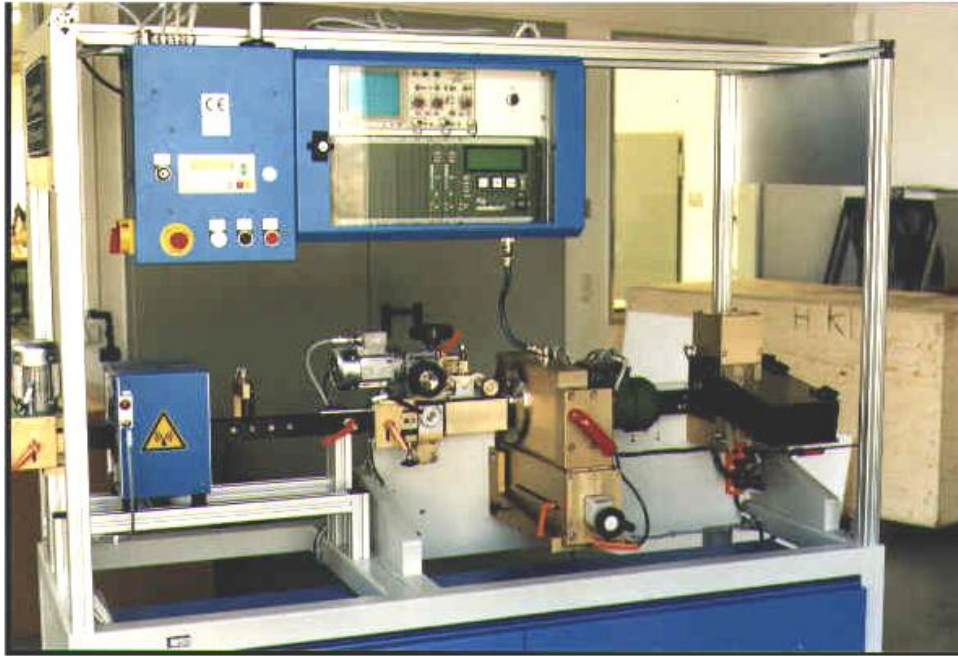
Feed, demag coil, driving rollers, rotating head eddyscan ® H63 with height-adjustable maintenance slide, lockable NOK parts chute, OK parts discharge.
