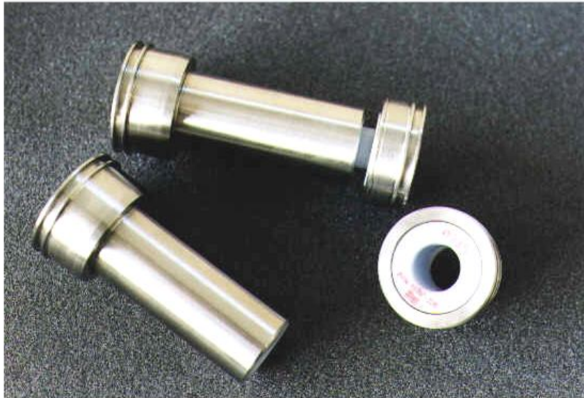
Easy change-over to different parts diameters by exchangeable guide tubes.
