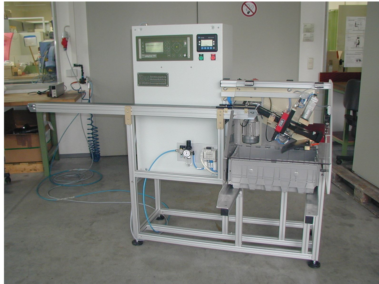
Front view of the test system with frame, PLC and test instrument eddyliner® P , conveyor belt, sorting station and marking station.
